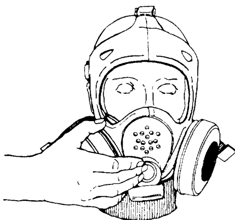
Figure 6-4.-Correcting sticking outlet valve with cover partially removed.
